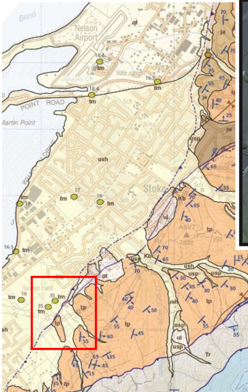
Blind reverse faults beneath alluvial cover
