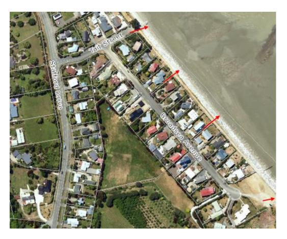
It was suggested that additional stormwater drains could be laid down the two alleyways off Broadsea Ave to improve drainage off the street.
